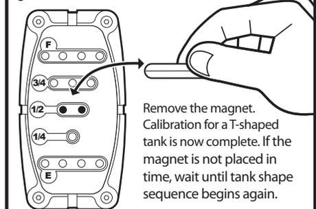
Remove the magnet. Calibration for a T-shaped tank is now complete. If the magnet is not placed in time, wait until tank shape sequence begins again.
