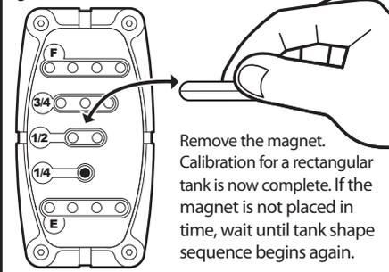
Remove the magnet. Calibration for a rectangular tank is now complete. If the magnet is not placed in time, wait until tank shape sequence begins again.
