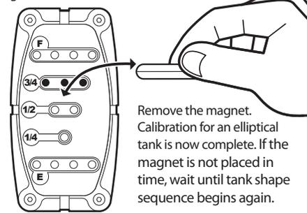
Remove the magnet. Calibration for an elliptical tank is now complete. If the magnet is not placed in time, wait until tank shape sequence begins again.
