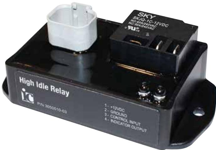
The Innovative Controls Inc. model 3050510-03 High Idle Relay is used to monitor the vehicle battery voltage and energize a relay when a low voltage condition is detected. The relay is typically used to increase the engine idle speed so that the alternator can recover the battery voltage. The High Idle Relay is a fully potted module that is suitable for automotive applications.
