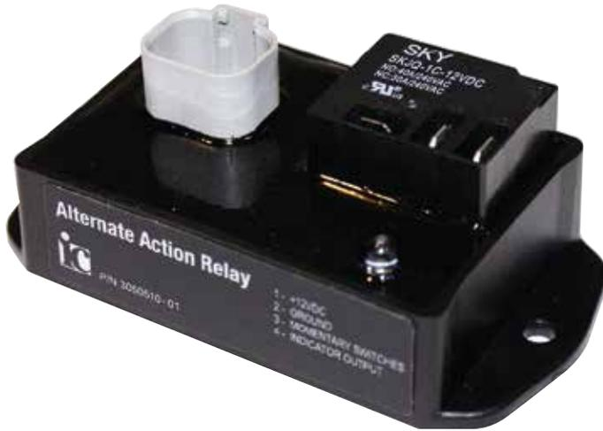
Innovative Controls Inc. 3050510 Alternate Action Relays are used to remotely control a load by momentarily switching the input to ground. The load is controlled by a 30 amp single pole, double throw relay with integral 1/4" quick connect terminals. The Alternate Action Relay is ideal for multiway switching applications where more than one switch is used to control a load.
